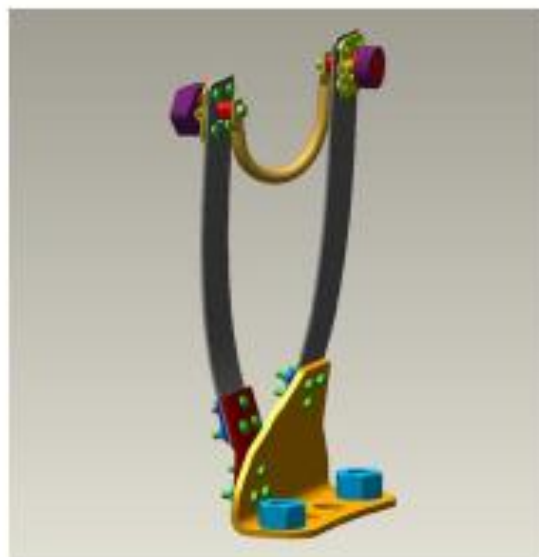
Figure 2-5: LCTU between blades and nacelle chassis
